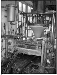
Machine for printing the design on plates and bowls.
