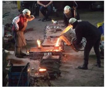
The church bells are cast slightly oversize from bell metal (77% copper and 23% tin) costing £10K/tonne. This gives a true attractive harmonic sound. Tuning is done by removing metal from the inner profile using trial and error method. Tested using a mix of old and modern methods a tuning fork/critical ear and a frequency generator.
